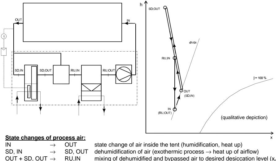
mixing of dehumidified and bypassed air to desired desiccation level  $(x_{IN})$  cooling of air down to desired supply temperature  $(t_{IN})$
