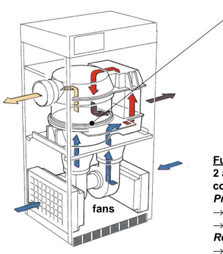
Sorption rotor: composed of large number of small channels impregnated with sorptive agent
